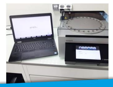
Analis acquires all data in real time. USP <1062> plots for tablet characterization are integrated into STYL'One Evo software. Manufacturability profiles (tablet breaking force vs compression force) and tabletability profiles (tensile strength vs pressure) are readily available. Compressibility and compactibility profiles can be used when powder true density is known. The user can also build customized plots and reports. As a result, Analis expedites research projects.
